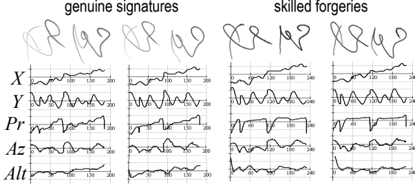
Figure 1. Off-line (images) and on-line (signals) representation of signatures.
